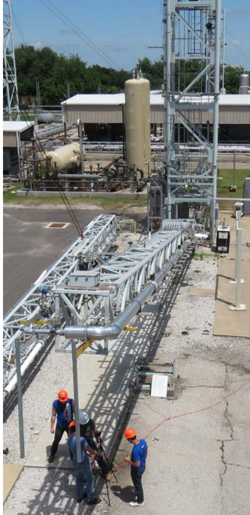
Figure 3. View of 2-in. Gas/Oil/Water Flow Loop
